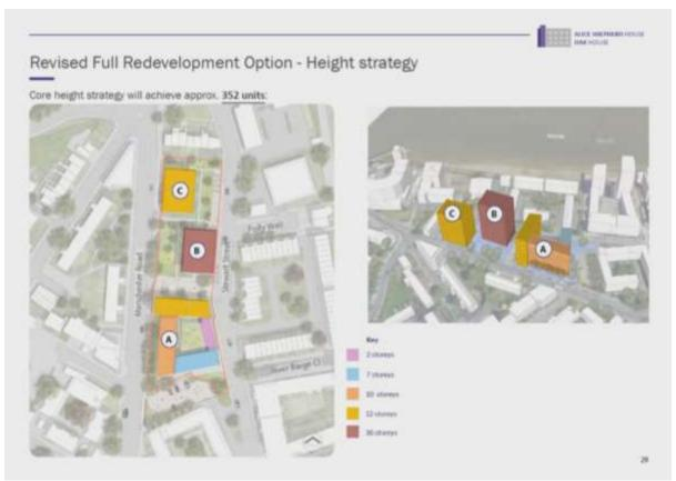
5.19 In this design Block C is 12 storeys, Block B 16 storeys and Block A is 2 storeys (pink), 7 storeys (blue), 10 storeys (orange) and 12 storeys (yellow). The higher part of Block A has been placed on the North side so it might not be possible
